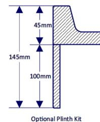
All measurement stated in mm to tolerance of +/-5mm
