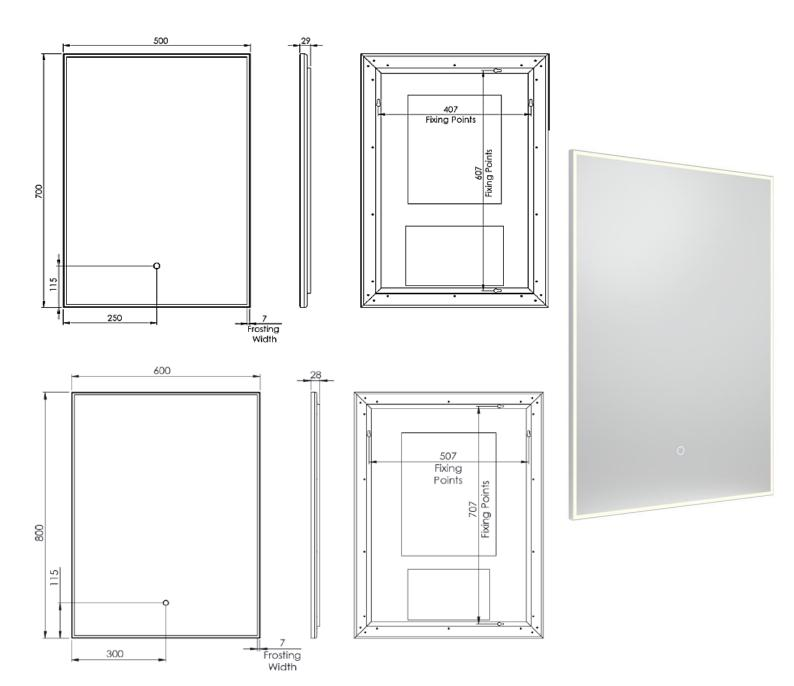
All Dimensions are in millimetres. | All Dimensions in mm have a tolerance of  $\pm$  5mmThe information contained on this page was correct at date of issue. Fitting dimensions are provided as a guide only. Some variation may occur due to manufacturing tolerances. We pursue a policy of continuing improvement in design and performance of our products and so reserve the right to change specifications without prior notice.
