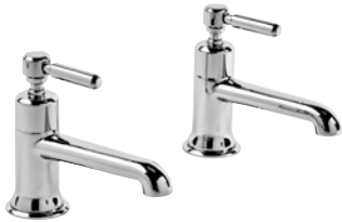
Marston Basin Taps Pair (Waste Not Included) See page 225 for more details on wastes Minimum recommended pressure 0.2bar 46(w) x 114(h) x 139(d)mm Chrome - TMS70
